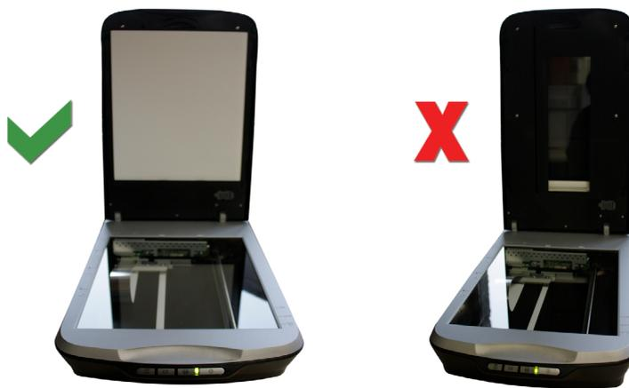
**2** Place your document face down on the scanner glass. Position the document so that the corner touches the point of the embossed arrow on the scanner bed. Close the scanner lid.
