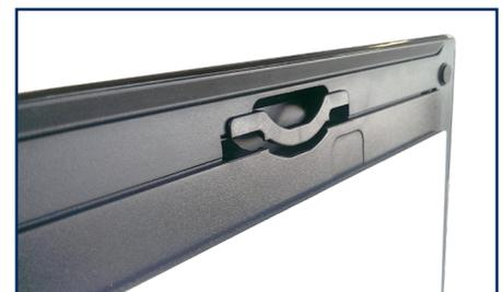
*The clip at the top of the inner cover which secures it to the underside of the scanner lid*
